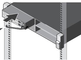
Beginning from the top, install the sled(s) into the enclosure, from left to right.
